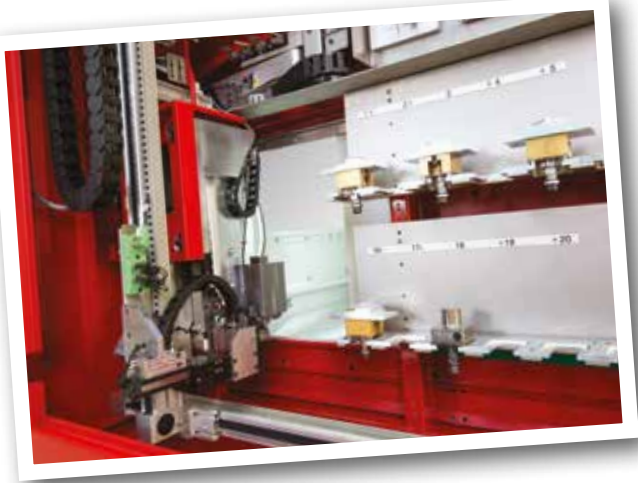
<< Figure 2: KERN workpiece changer can accommodate 30 workpieces and will pay for itself in under 12 months. Figures courtesy of KERN Microtechnik GmbH. >>
