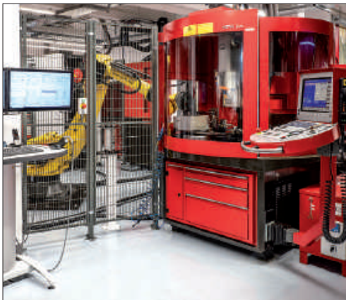
Kern Microtechnik integrated a robot cell in their shop; each of the four machining centers has a utilized capacity of 94%
