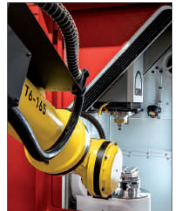
The complex control of the cell is done by the process control system "WorkShopManager"; among others, the system runs an articulated robot which loads and unloads four machining centers
