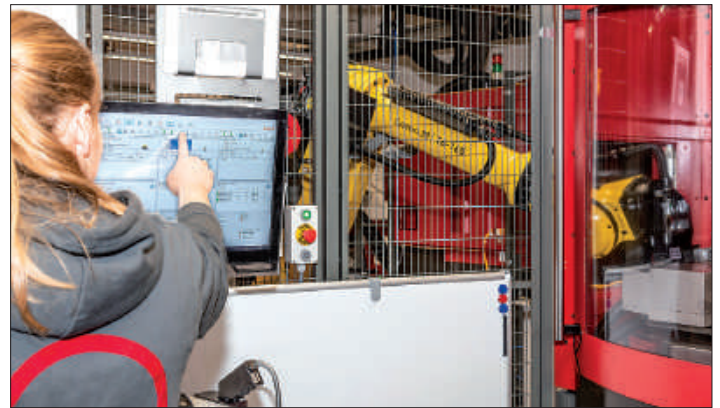
With a touch screen the WorkShopManager makes working with the robot cell easy; one qualified technician and one or two assistants are enough to run the robot cell and the four machining centers
