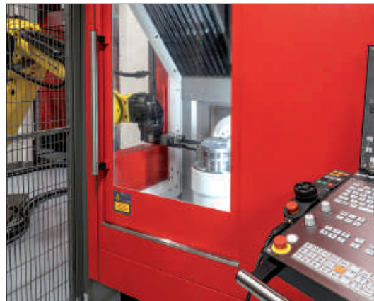
The complex control of the cell is done by the process control system "WorkShopManager"; among others, the system runs an articulated robot which loads and unloads four machining centers
